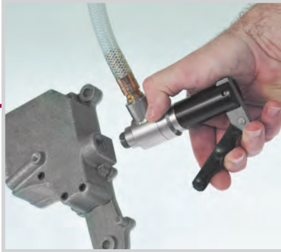
1 Squeeze lever to collapse the threaded collets
