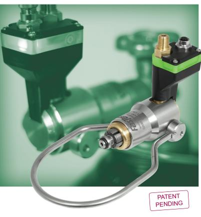
*FasTest's GT580 SMART System* provides instant visual confirmation that the connector has made a positive connection. Each connector uses an electrical output signal to relay connection status to a hub device that compiles the status of each individual connector. The hub analyzes each input and only allows the operator to begin the filling process once all connections have been properly made.
