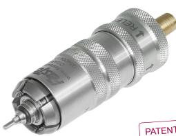
FasTest's G540 sleeve actuated Residual Pressure Valve (RPV) oxygen connector is simple to use with a no twist, no turn approach to filling. Simply connect onto your CGA 540 RPV valve and lock into place with a forward movement of the sleeve and you are ready to fill the medical or industrial oxygen cylinder in a matter of seconds.
