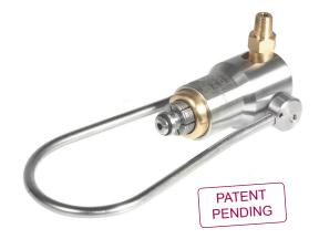
FasTest's G590 gas connector is simple to use with a no twist, no turn approach to filling. Simply connect onto your CGA 590 valve and lock into place with a forward movement of the bail handle roller actuator and you are ready to fill the cylinder in a matter of seconds.
