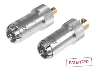
FasTest's G540 sleeve actuated oxygen connector is simple to use with a no twist, no turn approach to filling. Simply connect onto your CGA 540 valve and lock into place with a forward movement of the sleeve and you are ready to fill the medical or industrial oxygen cylinder in a matter of seconds.
