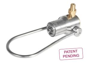
FasTest's G540 gas connector is simple to use with a no twist, no turn approach to filling. Simply connect onto your CGA 540 valve and lock into place with a forward movement of the bail handle roller actuator and you are ready to fill the oxygen cylinder in a matter of seconds.
