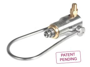
FasTest's G580 gas connector is simple to use with a no twist, no turn approach to filling. Simply connect onto your CGA 580 valve and lock into place with a forward movement of the bail handle roller actuator and you are ready to fill the cylinder in a matter of seconds.
