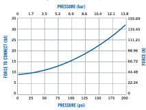
These graphs are intended to give you a general idea of the performance capabilities of each product line. Contact CPC for flow of a particular coupling combination.
